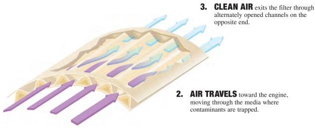
**DIRTY AIR** enters the Channel Flow filter through alternately opened channels on the intake side.
